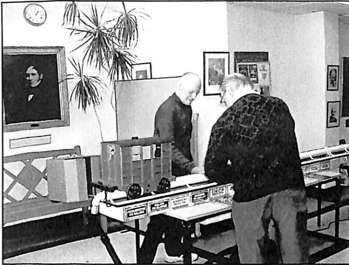
Norman Langridge demonstrates a scale model of Brunel's South Devon Atmospheric Railway in the foyer, during the Conference. The carriage on the left moves along the white tube from end to end.
