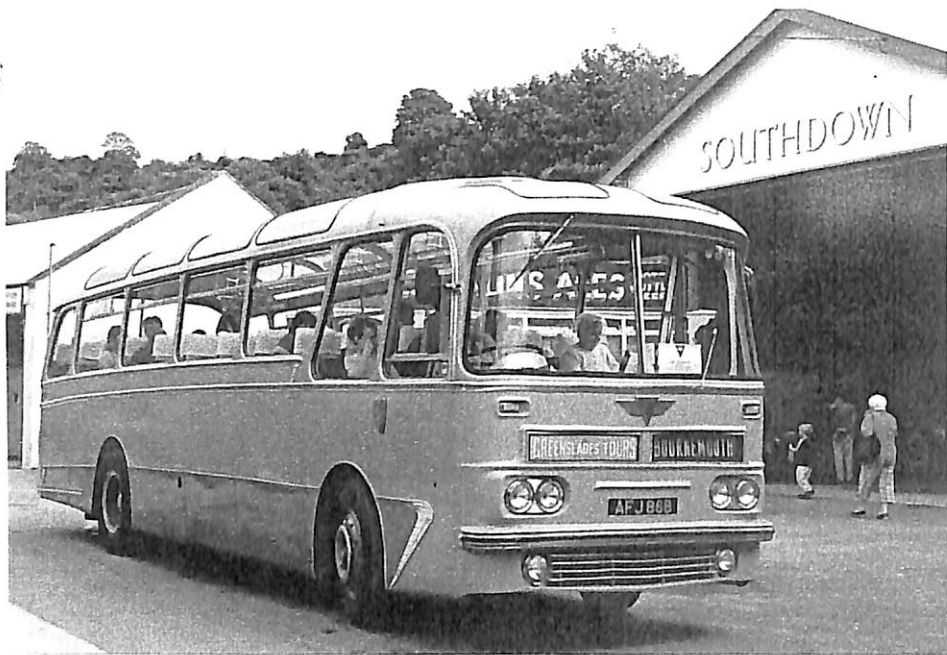
A 1964 A.E.C. Reliance coach with a 7' 6" Harrington 41 seat body for Greenslades Tours of Exeter, seen at the Amberley Working Museum
