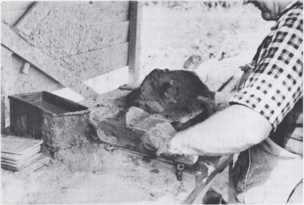
PLATE I Brick moulding using the strike
