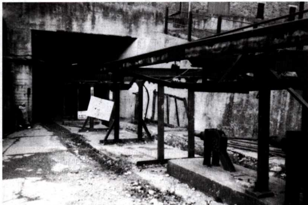
Fig. 4 Aerial cableway connecting Brightling Mine with the Mountfield Works, emerging from the mine at Brightling, taken in 1988 (W.R. Crawshaw)
