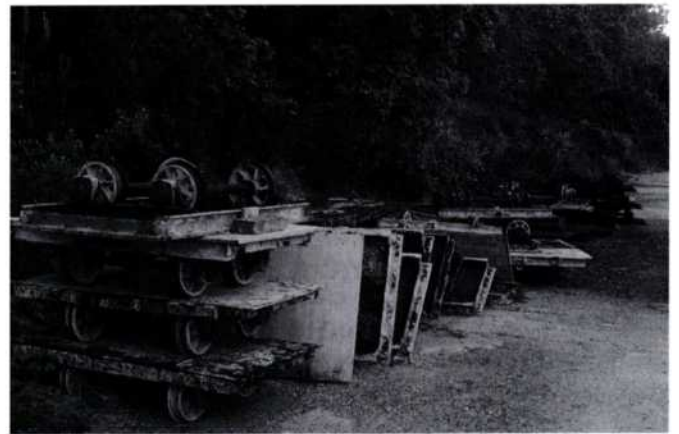
Fig. 5 Bogies used for brick transportation on 2 ft. 6 in. gauge Works railway. Photo: Brian Austen
