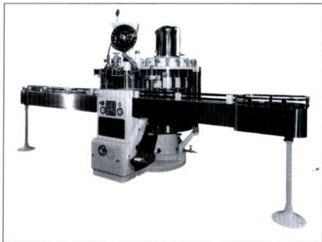
Fig. 6 The largest in the range; the Riley 18 head Automatic Bottling Machine.
